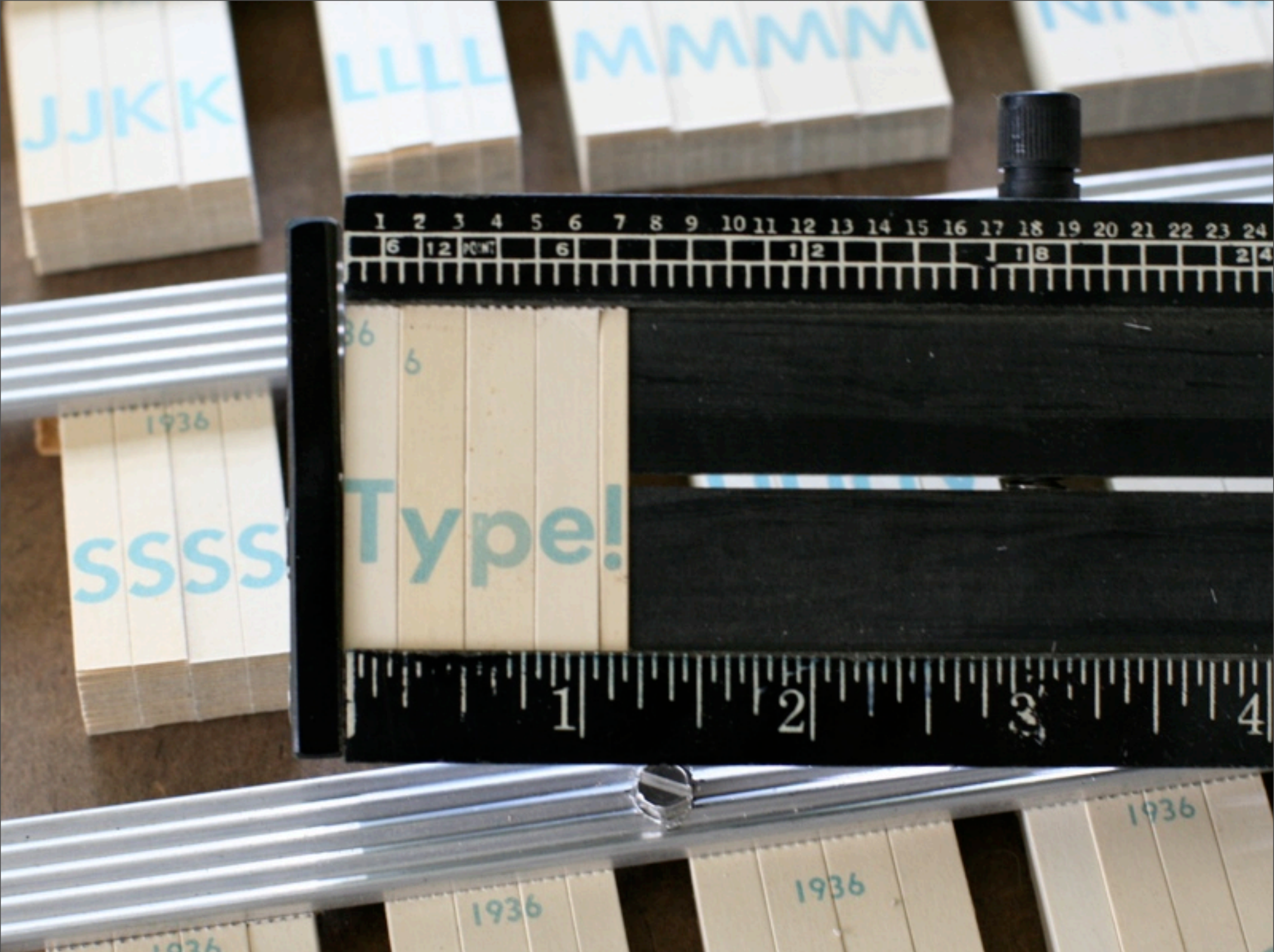
and assembled characters into words with the black side down on a sort of casting stick
